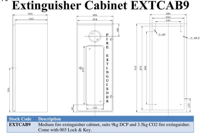
Please note: This cabinet has been phosphate and red powder coating treated, with high UV protection and anticorrosion level.
